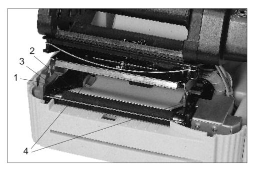
Fig. 6-3 Feeding Labels through Adjustable Label Edge Guides
